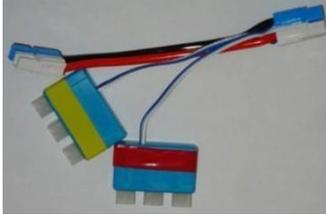
Track Bus Feeder Cables (soldered to bus)
