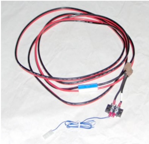
8 foot bus wire using 12v red/black DC power cable. The left end attaches to the cable from the terminal / splitter block.
