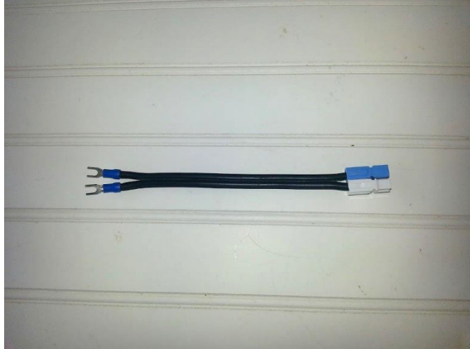
Figure 2 - Single Bus Power Source Cable
