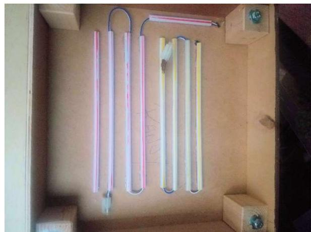
This photograph highlights Vic’s use of plastic drinking straws to provide the stress relief on the feeder. The feeder wires are fed into the straws in the manner shown, which prevents any stress on the Unijoiner connection.
