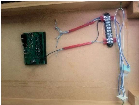
This photograph shows Vic’s use of Cup Hooks, inserted into the side of his module, to provide some stress relief for the feeder wires.
