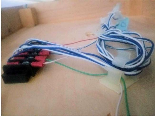
*Figure 1 - Adhesive-backed Plastic Clips
