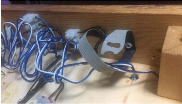
The Velcro strip is screwed into the side of the module using a sheet metal screw. This photo shows the Velcro unfastened and the wires loose.
