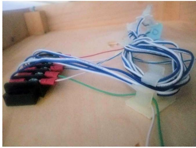
The use of the Adhesive-backed Plastic Clips from a different angle. Note that Vic (and *North Texas T-Trak*) also use colored bread bag tags to mark the various feeder wires – **BLUE** for the front track, and **WHITE** for the rear track. In the case of a Junction Module, the WHITE tags are also marked “L” and “R” (for Left rear track, and Right rear track respectively).
