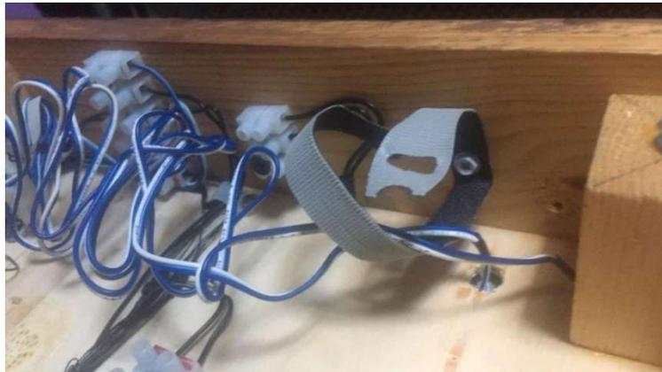
*Figure 8 - Velcro Cable Straps
