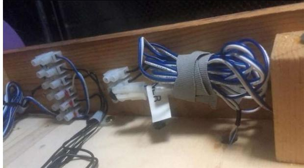
This photograph shows the Velcro strap fastened around the feeder wires.
