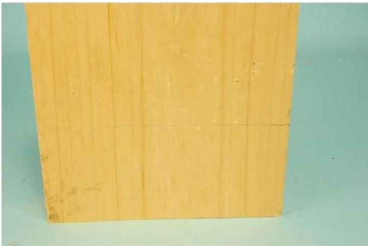
**Mark a line 1-1/2" from the edge perpendicular to the "face".**
