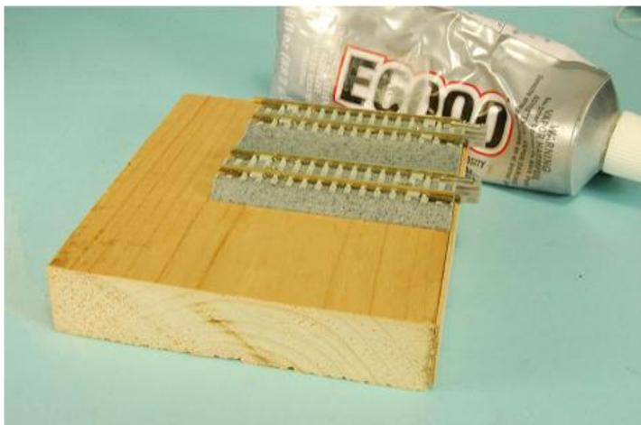
**Glue the 1/32 thick wood to the face of the block of wood.**
