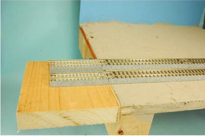
**Build a left and right and the track is easy to align on the module.**
